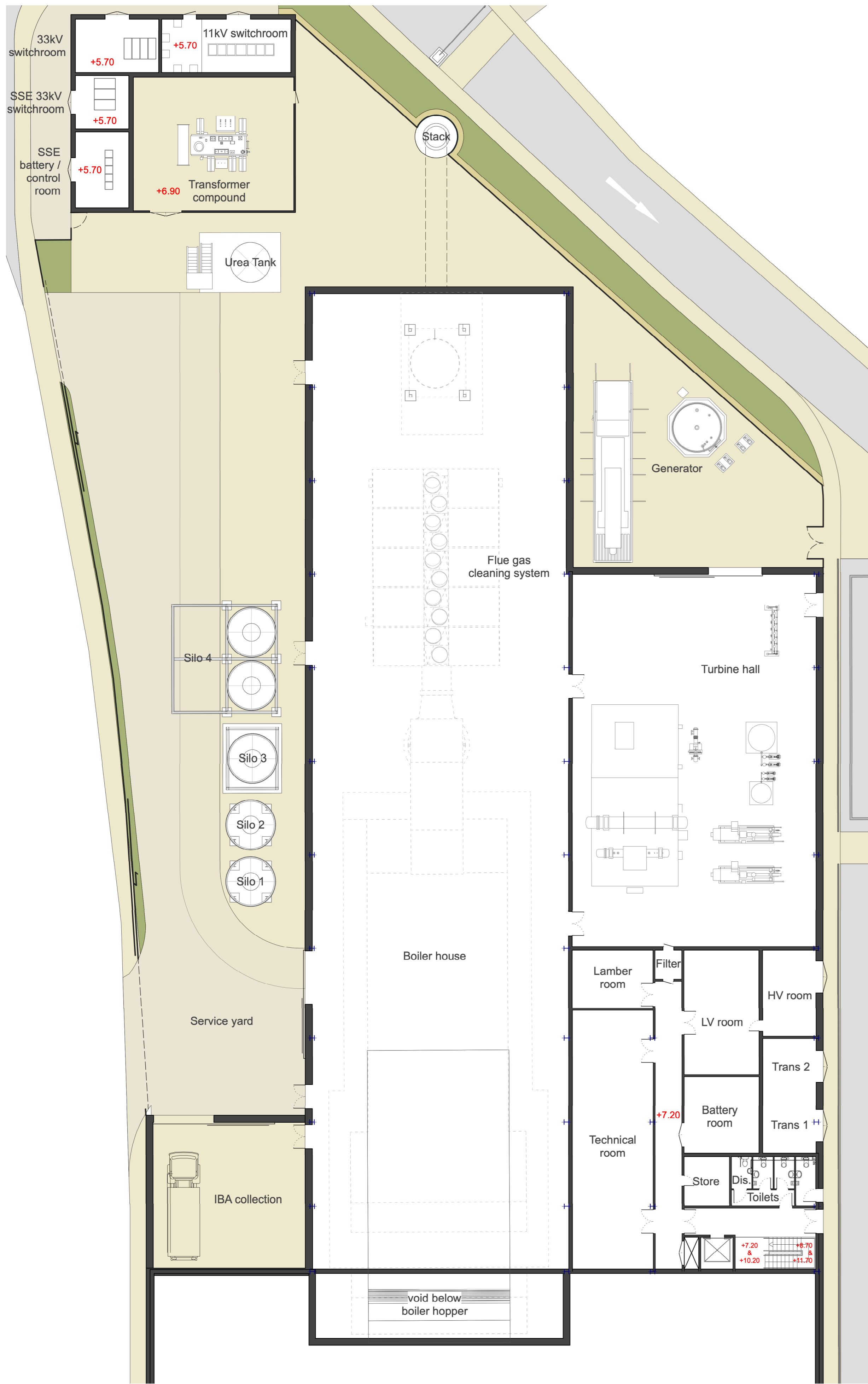
01 Proposed Ground Floor Plan 1:200 @ A1 / 1:400 @ A3
